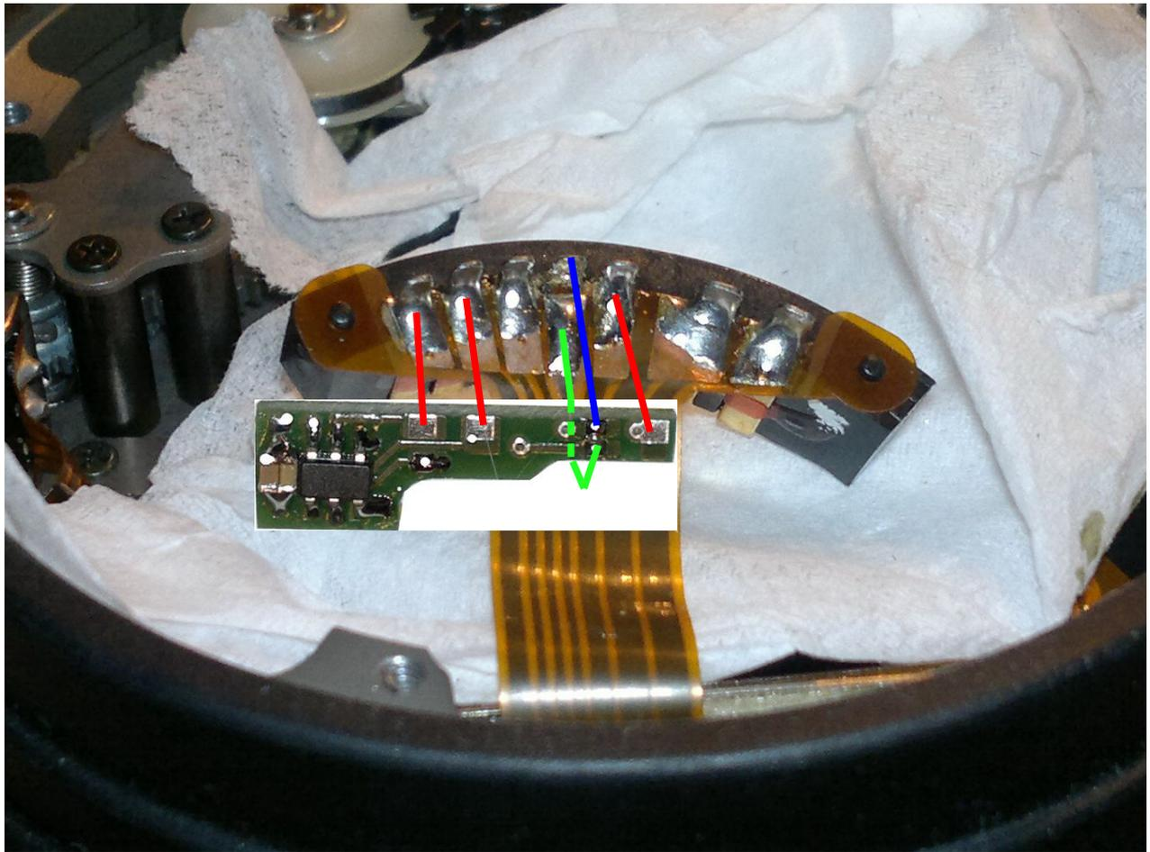
4. Board needs to be connected as per image above. Dout input to board (marked by blue line) needs to be isolated from Dout output from board (marked by green line) Dout output from board is very near Dout input to board so pay attention to not short them. Dout output needs to be connected to flex cable solder pad by wire which is supplied with board or can be connected by solder bridge.
