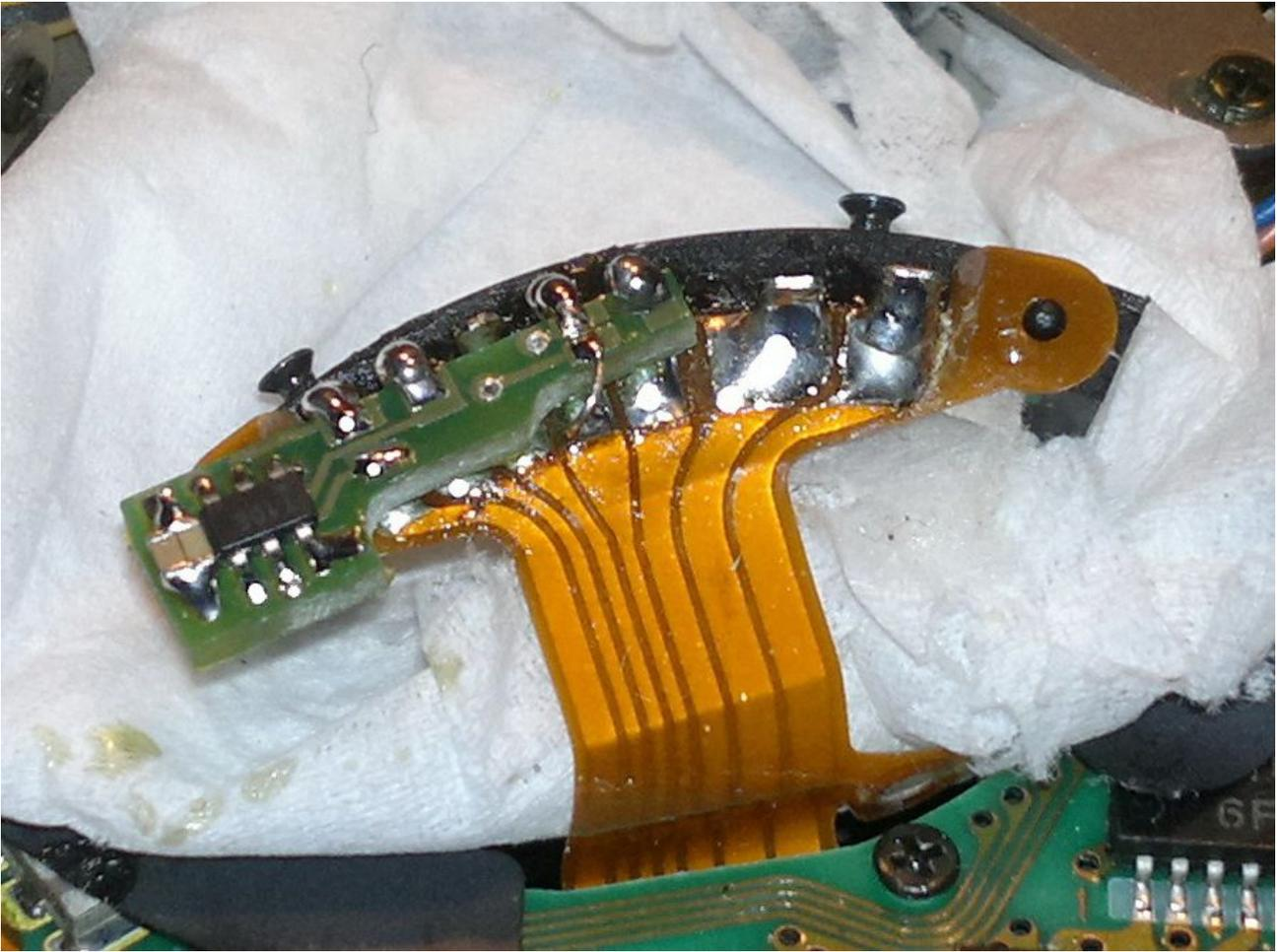
5. Model B is designed to horizontal installation as you can see on image. Also there is clearly visible how are solder pads on board soldered to individual pins as per diagram in step 4. Note Dout output from board which is connected by tiny wire, which is part of package with board, to flex cable solder pad. Again make sure that Dout input to board and Dout output from board are not shorted by solder or by any other way. Check this by multimeter to be sure.
