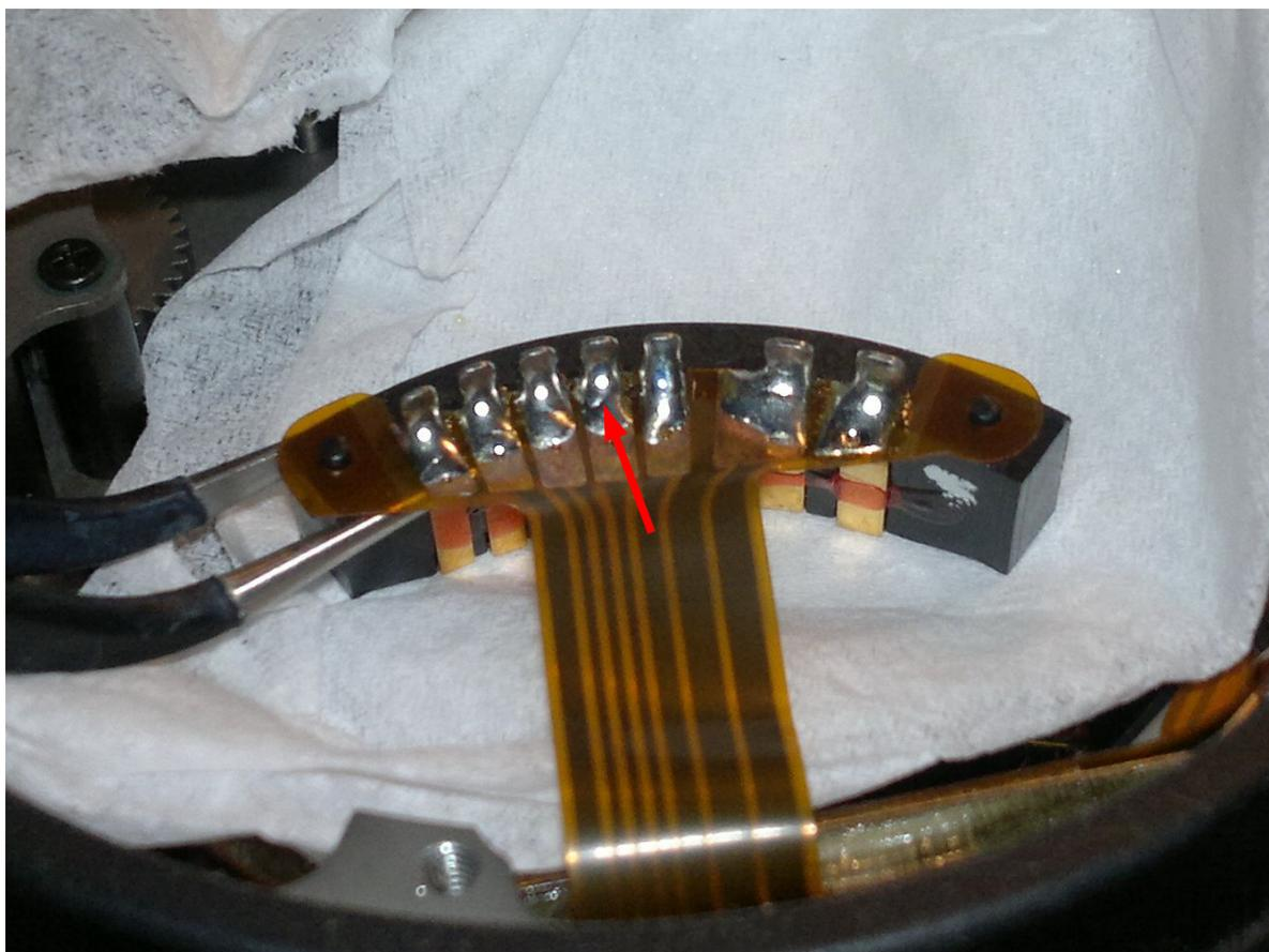
2. Remove solder from Dout pin (marked by red arrow). Use solder wick to remove it.
