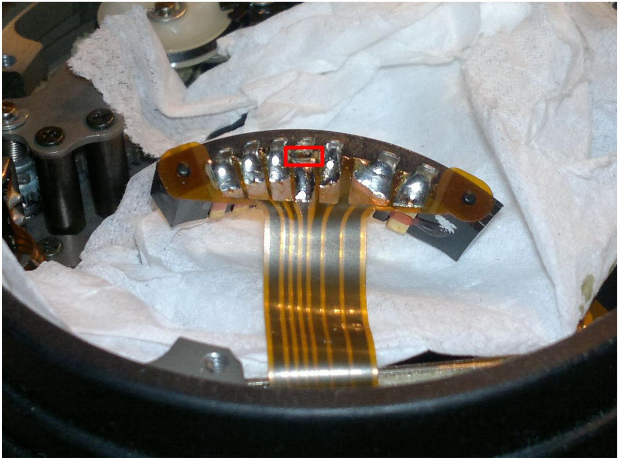
3. It is necessary to isolate pin and flex cable solder pad. To achieve this cut off 1mm of flex cable solder pad near pin. After this procedure there should be visible distance between solder pad and pin (highlighted by red rectangle).
